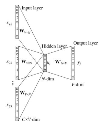
Figure 2.11: CBOW neural network architecture (Figure source: http://alexminnaar.com/word2vec-tutorial-part-i-the-skip-gram-model.html).
