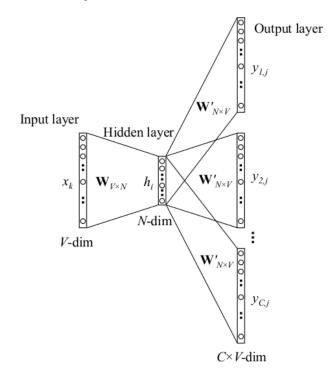
Figure 2.10: SG neural network architecture (Figure source: http://alexminnaar.com/word2vec-tutorial-part-i-the-skip-gram-model.html).
