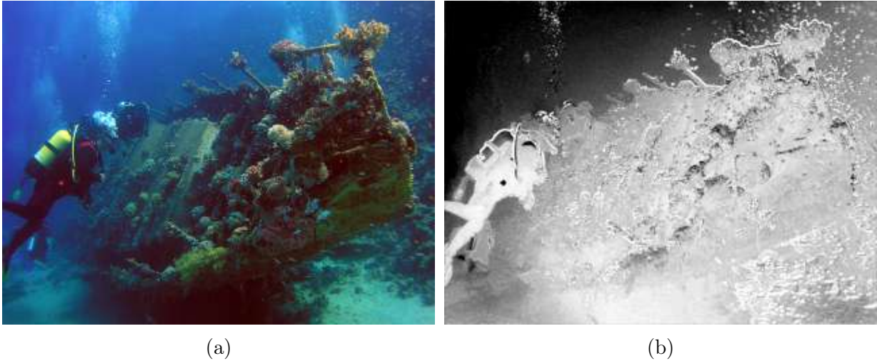
Figure 4.3: (a) an example of an underwater image; (b) the transmission map of the image on the left.
