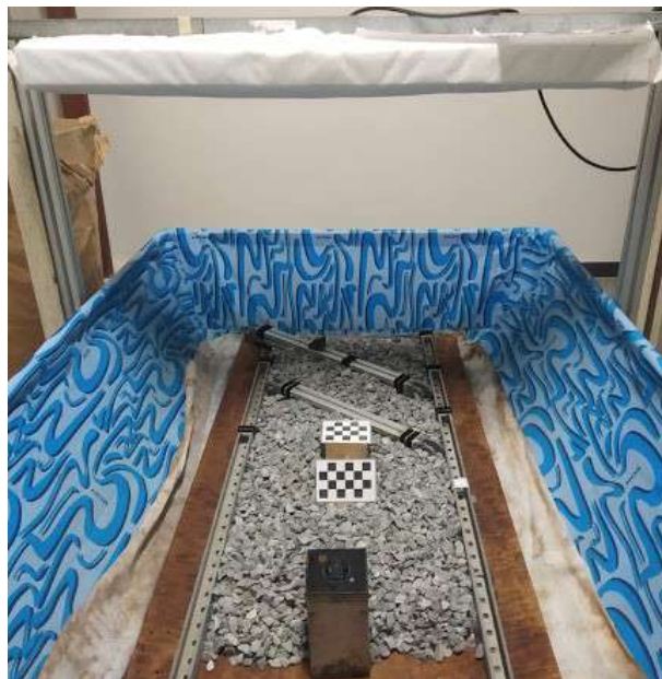
Figure 5.4: Setting up of the UVision19 dataset. It is possible to see the water tank, the calibration marks and the supports for the camera, the light source and the objects.
