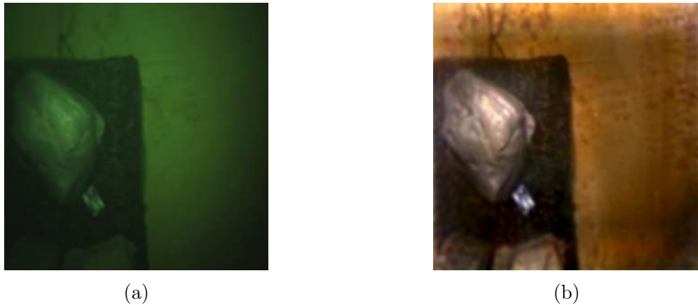
Figure 2.11: WaterGAN restoration result. Color-shifting was also removed, as we can see in (b). Images extracted from [31].
