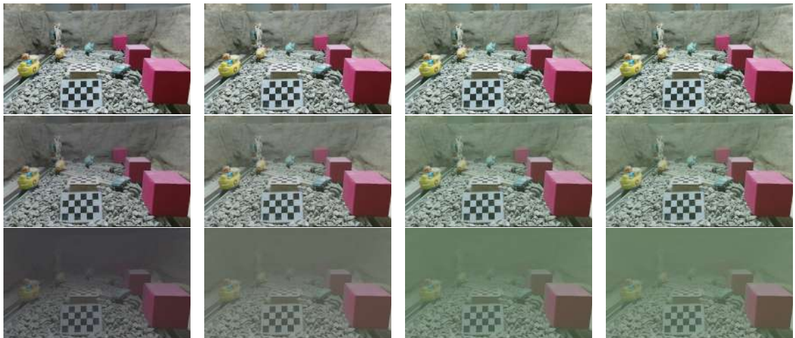
Figure 5.11: Kinect One synthetic images. Attenuation coefficients used from top to bottom rows: 0.244, 0.65, 2.07. These coefficients are displayed in Table 5.1, respectively referring to 600nm, 700nm and 800nm wavelengths. Approximated background light from left to right columns: clean water, 15g green tea, 20g green tea, 25g green tea.
