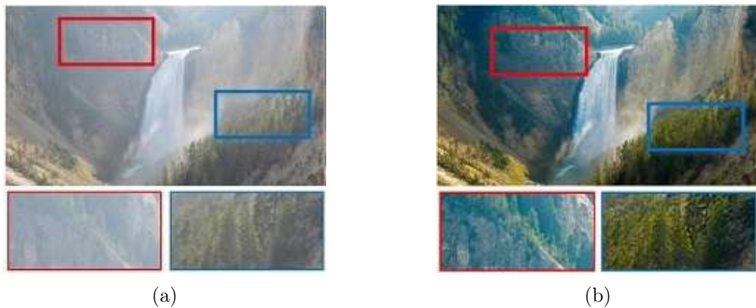
Figure 2.10: MSCNNDehazing result. Blue and red boxes zoom into detailed from the scene that were recovered during the restoration. Images extracted from [47].
