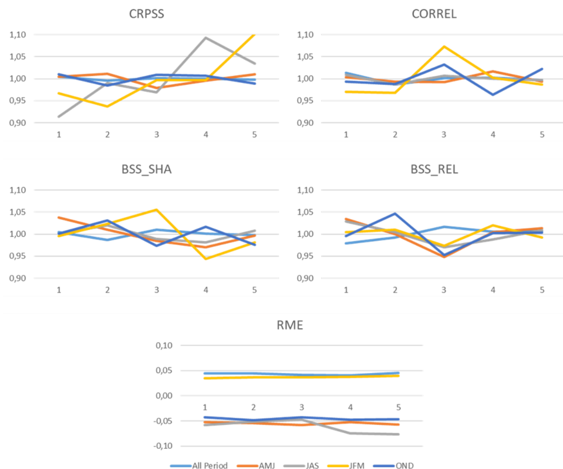
Figure 6.4– Evaluation of the five performance metrics, for the coupling time window of 30 days, the four first metrics the values are divided by the mean value, with different colors for the results considering the complete year and the seasons OND, JFM, AMJ, JAS; the x-axis represents the different coupling methods (1-Euclidean distance 15 days, 2-Euclidean distance 15 days, 3-Member-to-Member, 4-Volume last 15 days and 5-Volume last 30 days).
