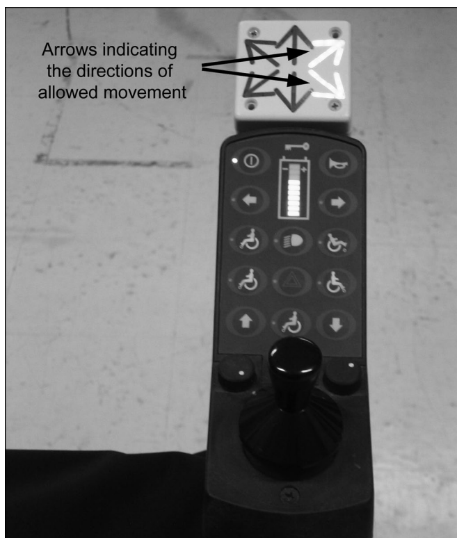
Figure 2. Joystick controller with indicator lights.
