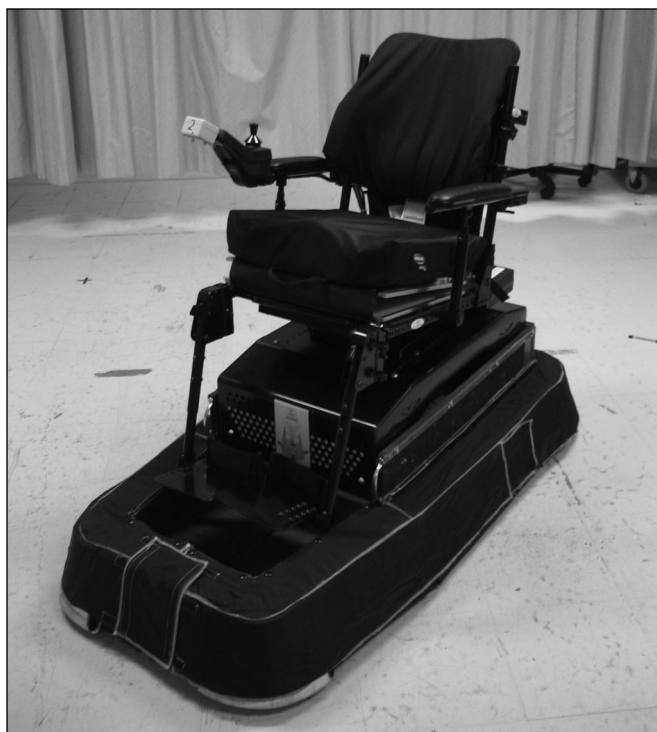
Figure 1. Anticollision power wheelchair.
