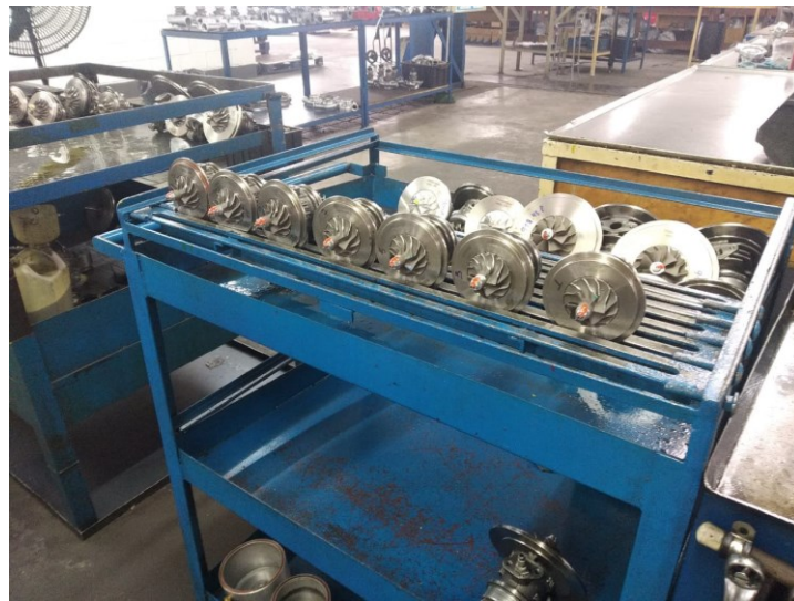
Figure 24 – The seven rotor-bearing sets after balancing
