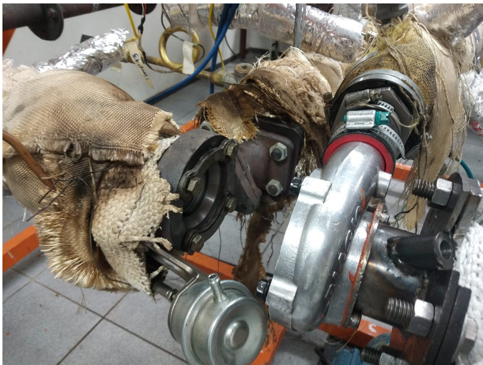
Figure 26 – Workbench with the AUT1000 compressor and turbine housing and without the rotor-bearing set
