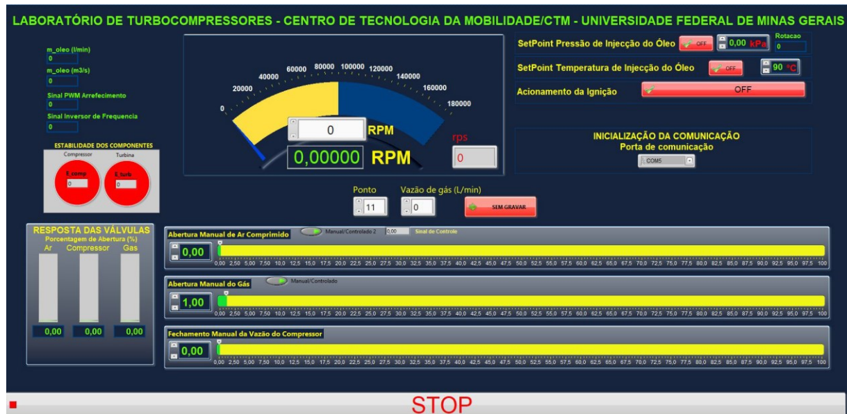
Figure 49 – Fluid pressure and temperature supervision interface.
