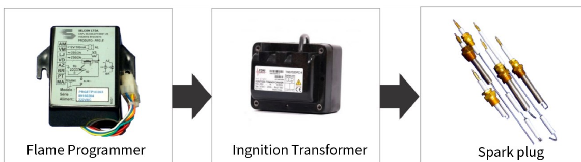
Figure 43 – Layout of the combustion ignition system
