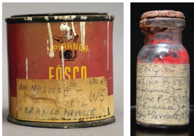
figure 7. Two examples of Oiticica studio paints. The can on the left bears a handwritten label indicating the use of amarello melilla, verde Betonol and branco Nivelle. While labeled côr H , the object with which this color is associated is not given. The glass vial on the right is labeled Invenções no. 34 and ingredients listed include vermelho P-5874 , vermelho P-5893 , nipagin and secante .
