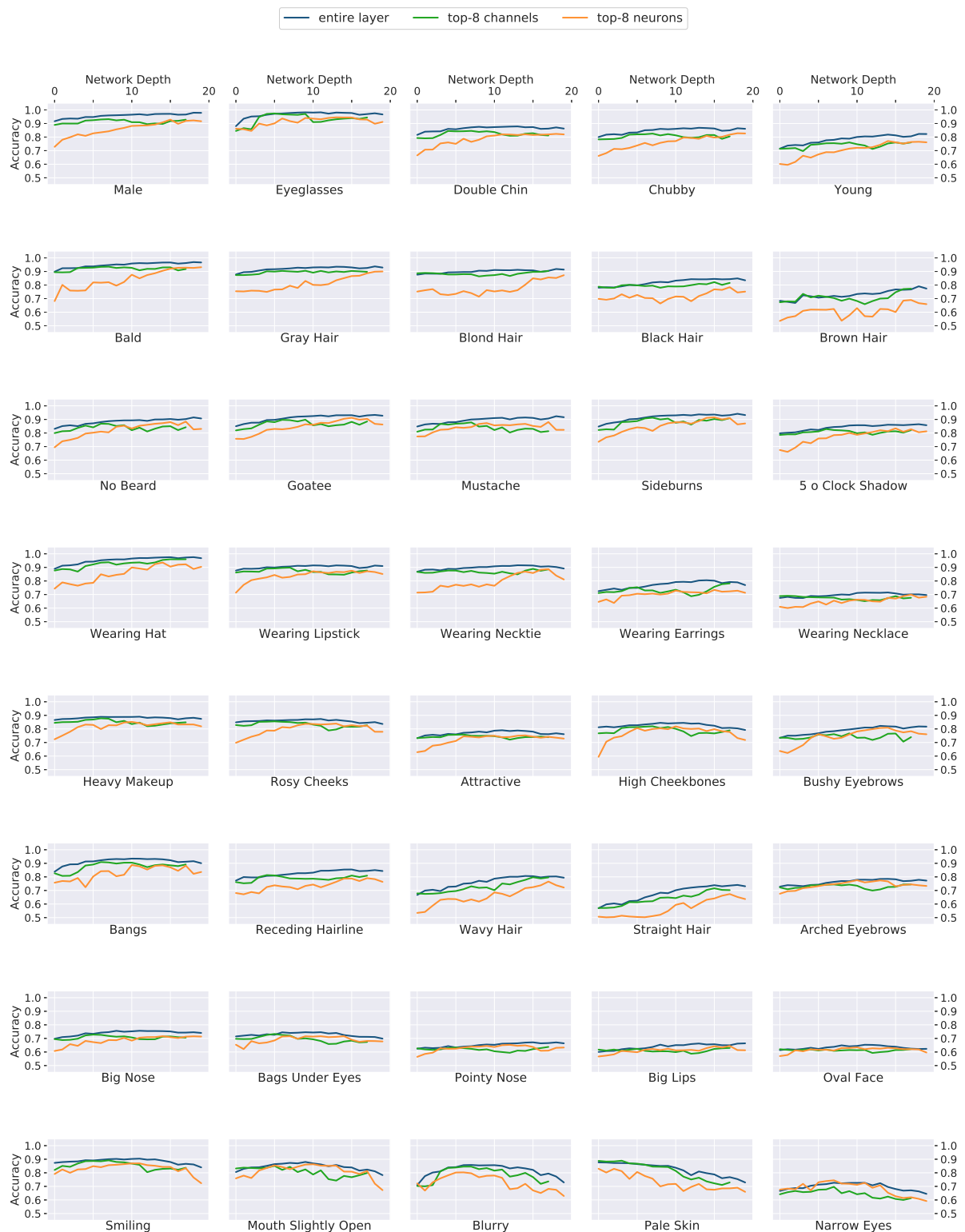
Figure 5.3: Attribute prediction accuracy over the depth of the VGG16 network. The blue curve measures the accuracy obtained by an attribute classifier that uses the entire layer response as its input. The green and orange curves replace the layer representation by a subset containing the eight top-scoring filters and neurons, respectively.
