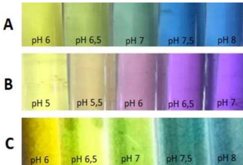
**Figure 1 - Standard colors of Bromothymol Blue and Bromocresol Purple at different pH.** (A) Buffered standard solutions from pH 6 to pH 8 containing 0.1% Bromothymol Blue. (B) Buffered standard solutions from pH 5 to pH 7 containing 0.1% Bromocresol Purple. (C) Buffered standard solutions from pH 6 to pH 8 containing 0.1% Bromothymol Blue and serum.
