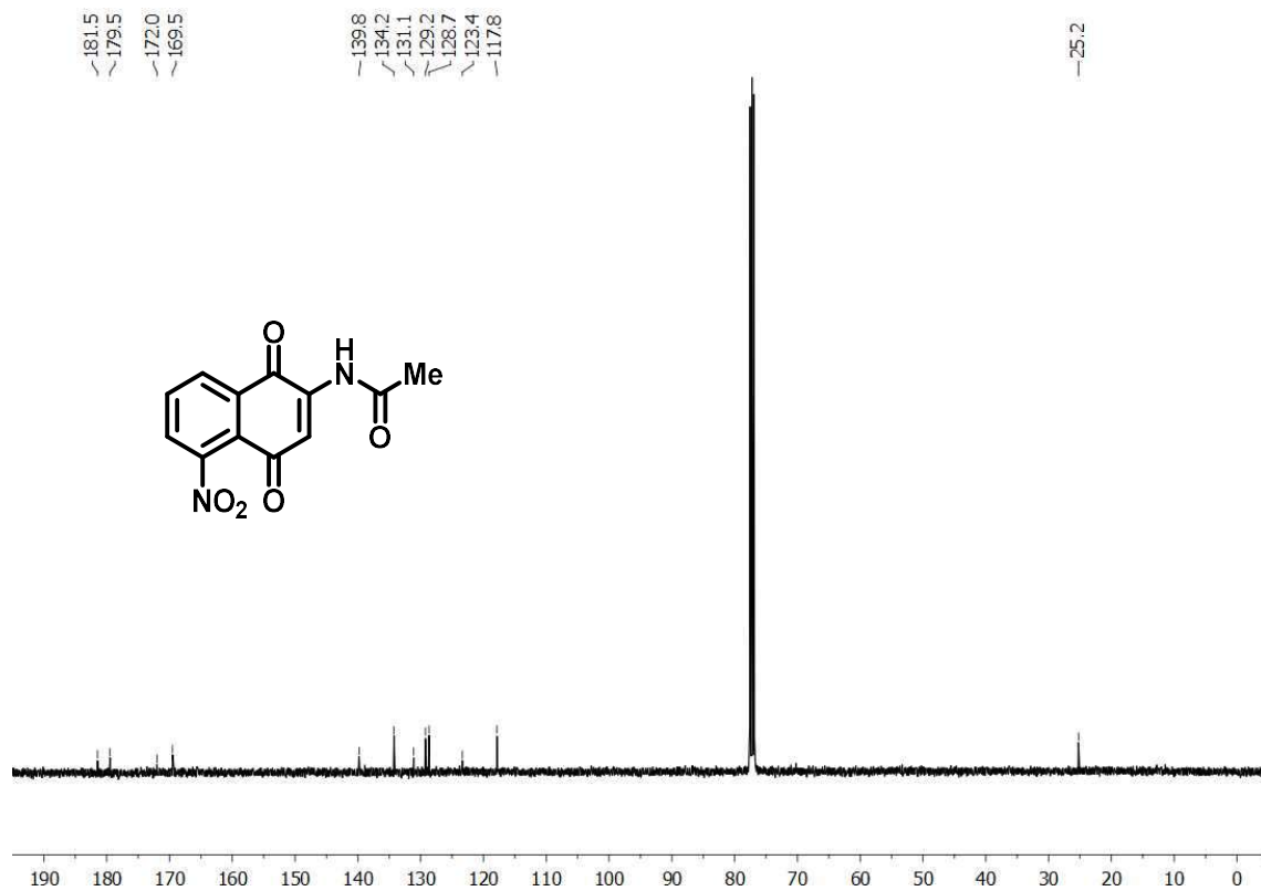
Figure A92. 13 C-NMR spectrum of compound 59b (CDCl 3 , 100 MHz).
