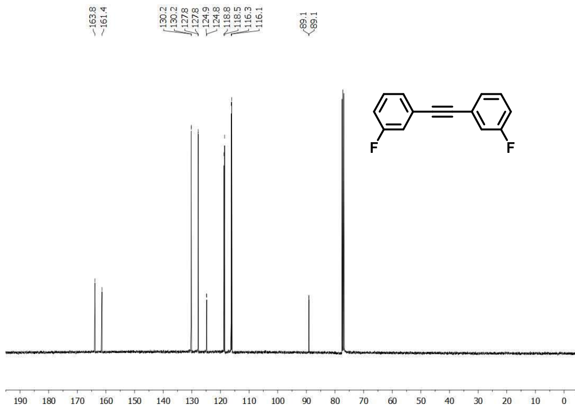
Figure A42. 13 C-NMR spectrum of compound 56p (CDCl 3 , 100 MHz).
