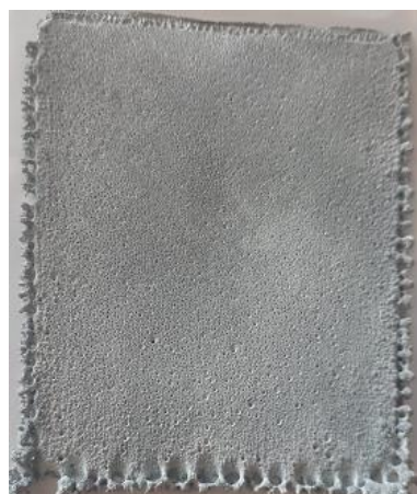
(e) 550Am^{-2} e [Mg^{+2}] = 15gL^{-1}
