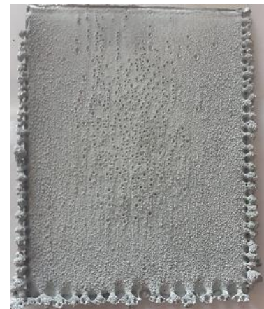
(c) 650Am^{-2} e [Mg^{+2}] = 1gL^{-1}
