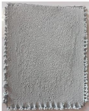
(b) 550Am^{-2} e [Mg^{+2}] = 1gL^{-1}
