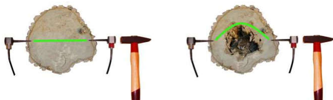
Figure 1. Stress waves principle, Fakopp (2012)
