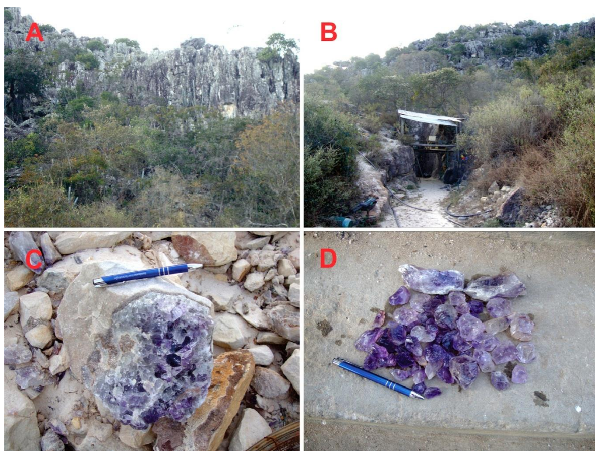
Figure 5.5: A) Ruiniform quartzites showing a vertical foliation which is typical in Tibério's mine. B) Aspect of the main pit that goes down to the vein being currently mined at around 30 m deep. C) Part of an amethyst vein in the host quartzite. D) Hand selected amethyst batch with deeper color.
