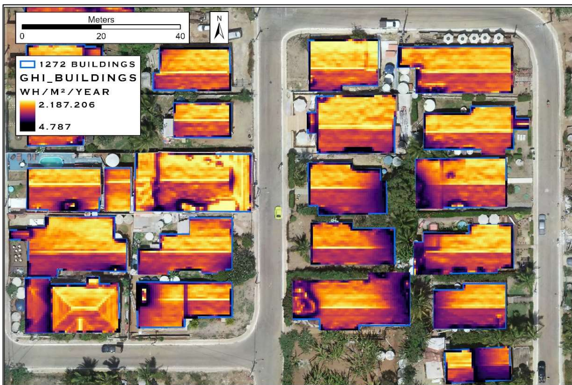
Figure 39. Irradiation data extracted by building vectors.
