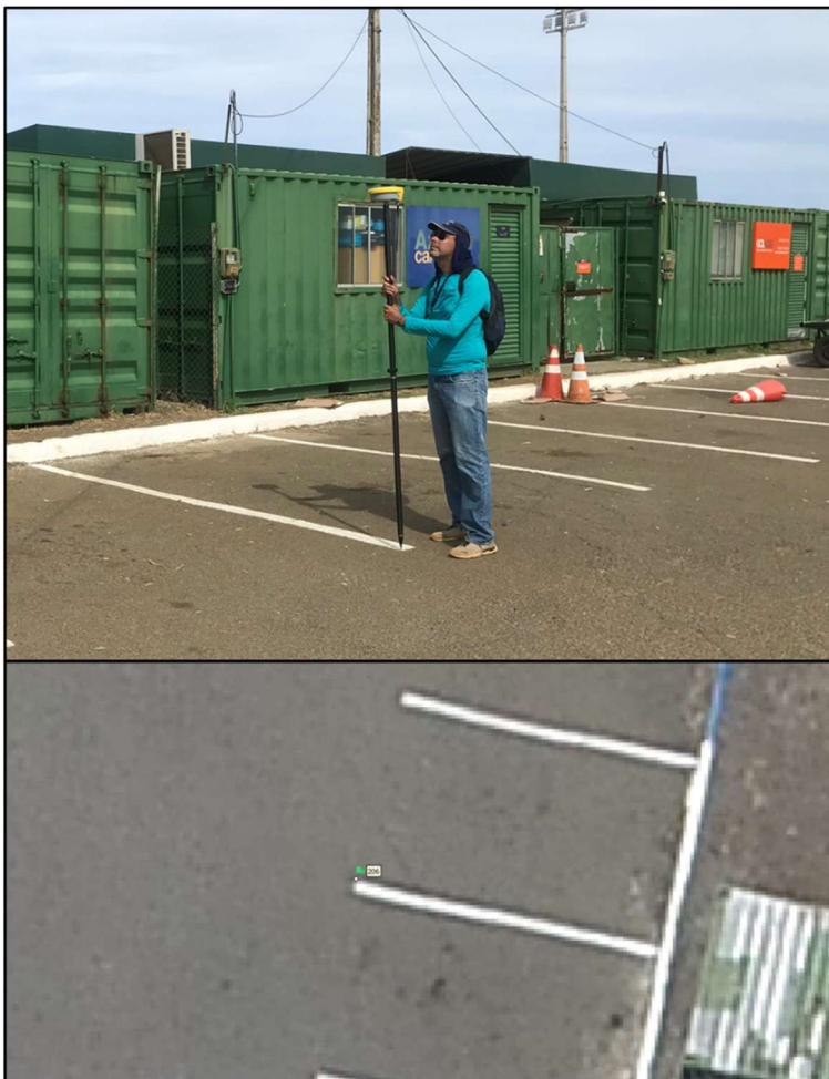
Figure 24. Up: GCP measured in a stripe painted on the floor (Professor Marcelo Nero). Down: Placing a marker on a photo.
