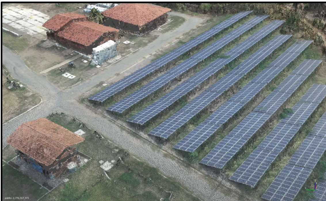
Figure 29. Dense point cloud representation of Noronha II PV Plant and sloping rooftop.
