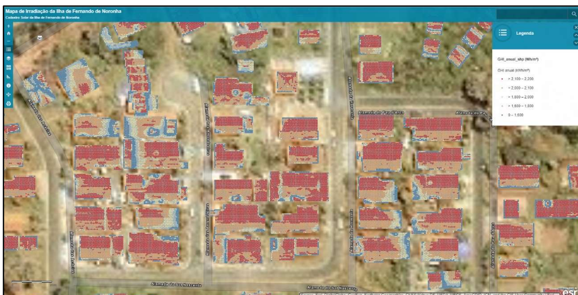
Figure 44. Web GIS platform. Zooming in will show the shapefile of points informing the annual GHI in rooftops.
