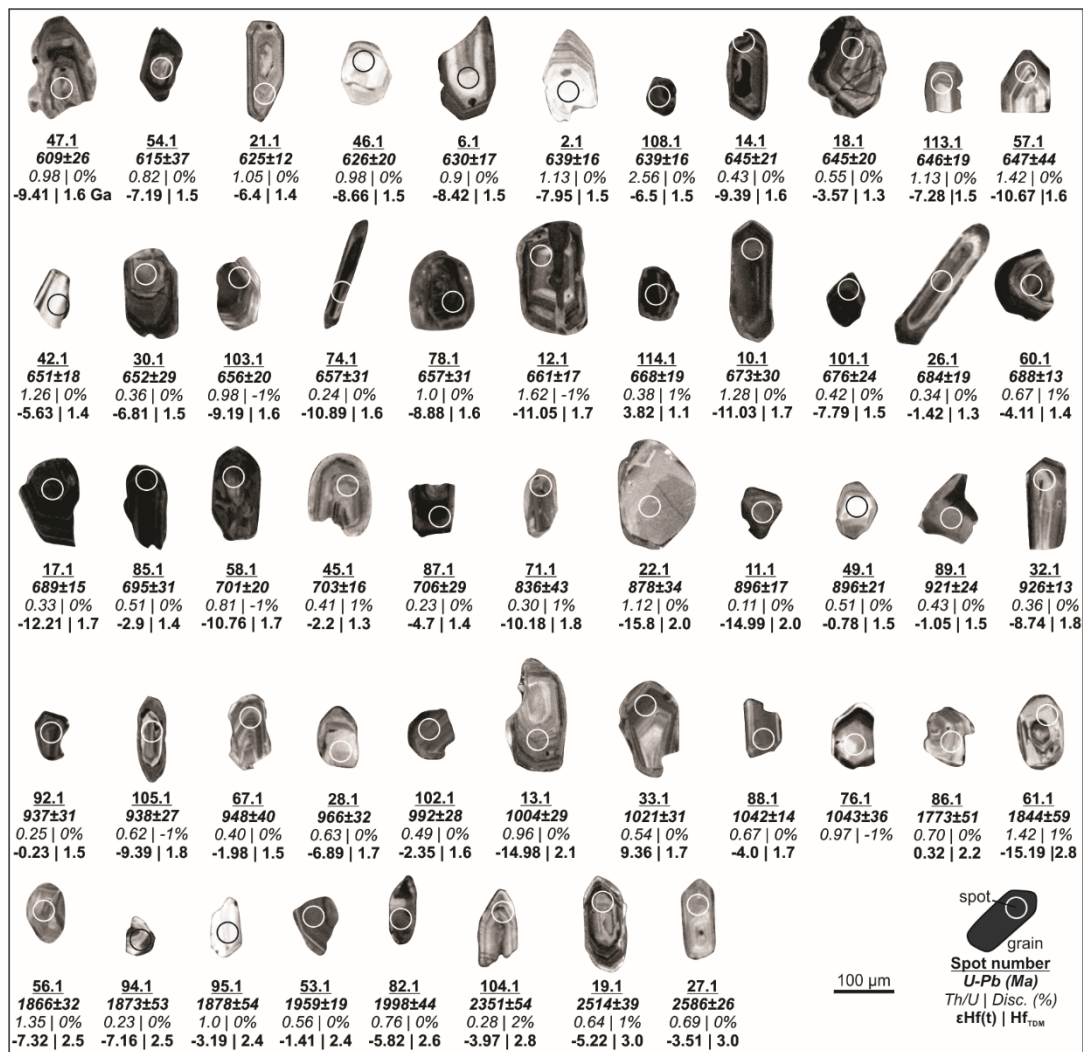
Figura 3.3– Selected cathodoluminescence images and spot placement for zircons grains from sample JK1. Quoted ages are ^{207}\text{Pb}/^{206}\text{Pb} dates for grains > 1.0 Ga and ^{206}\text{Pb}/^{238}\text{U} dates for grains < 1.0 Ga.
