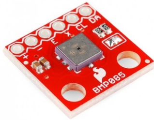
(c) BMP-085. Temperature sensor
