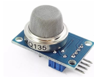
(b) MQ-135. Air quality sensor.
