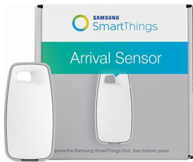
(a) SmartThings Arrival Sensor in format of Keychain used for presence recognition
