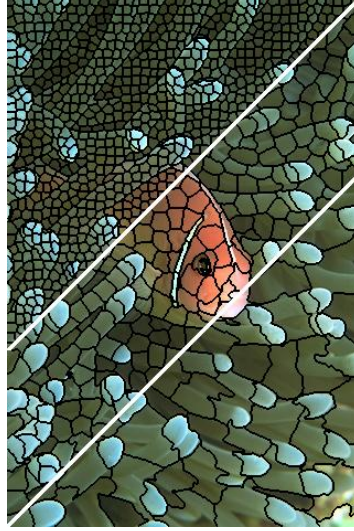
Figure 4.4: SLIC result image example with three different number of superpixels.
