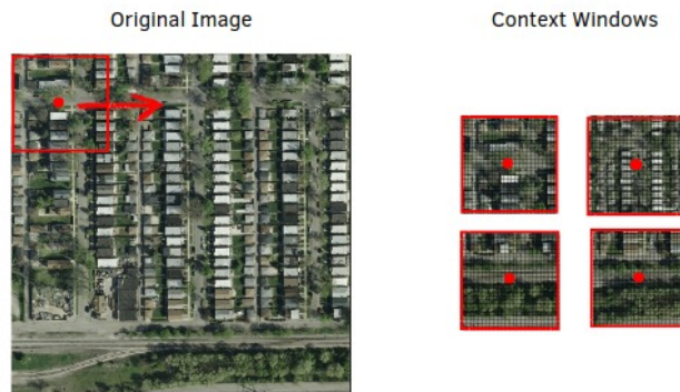
Figure 4.3: Illustration of context windows method for a pixel. It is replicated for all pixels in an image. The red square slides pixel by pixel over the entire image.
