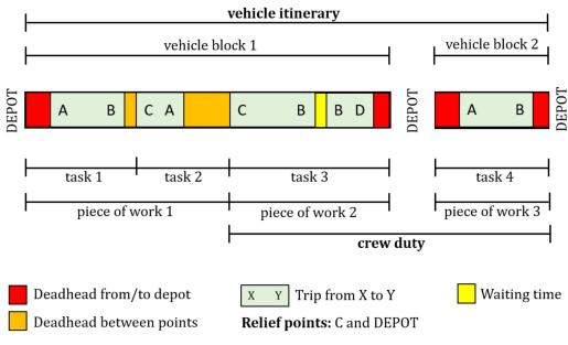
Figure 3.1: Example of vehicle itinerary and its crew duty.
