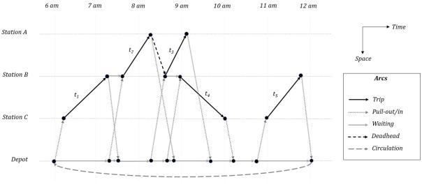
Figure 3.2: Time-space network layer for the MDVSP.
