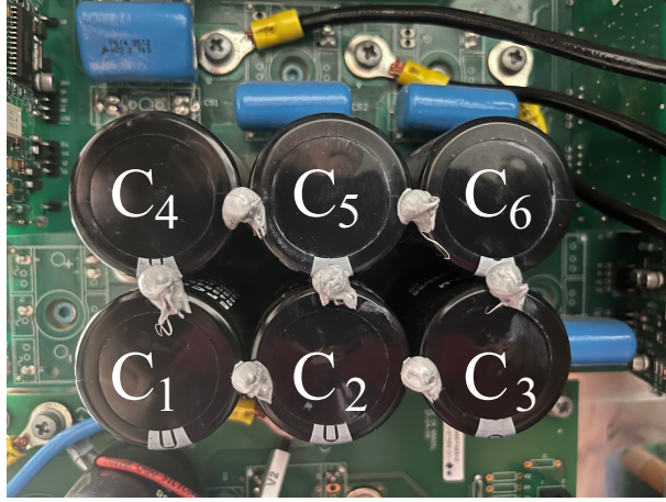
Figure 59 – Capacitor bank of INV1 with the specification of C_1 to C_6 .
