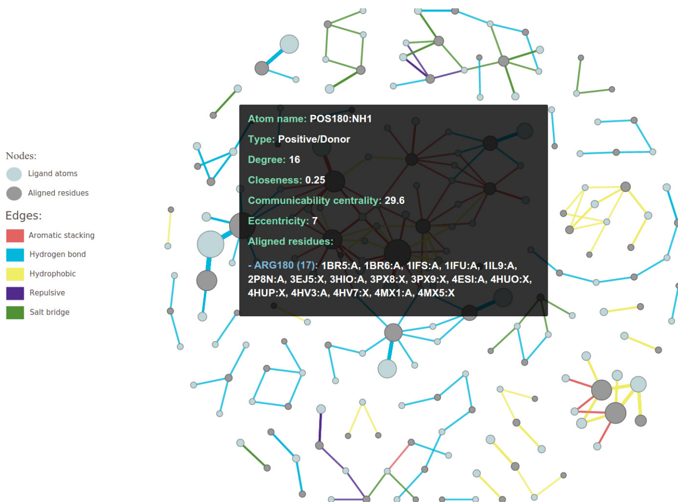
Figure B.4: Details on demand. For every element of the graph, details can be obtained on demand by passing the mouse over it. In this example, we obtain node details by positioning the mouse over such node. The graph is from Ricin dataset.
