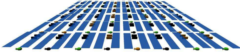
Figure 4.25. 64 instances of the environment during parallel training. For the turbines, green represents power generation mode. For turbines and sluices orange represents idling/slucing mode and black – offline mode.
