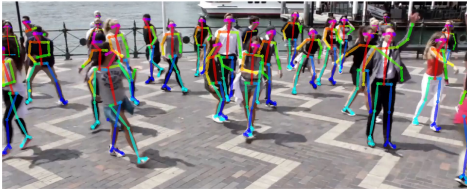
Figure 1.1: Example of skeletons extracted from an image. After extraction, the pose information is condensed in the graphs immune to background noise and lighting. Image extracted from [3].
