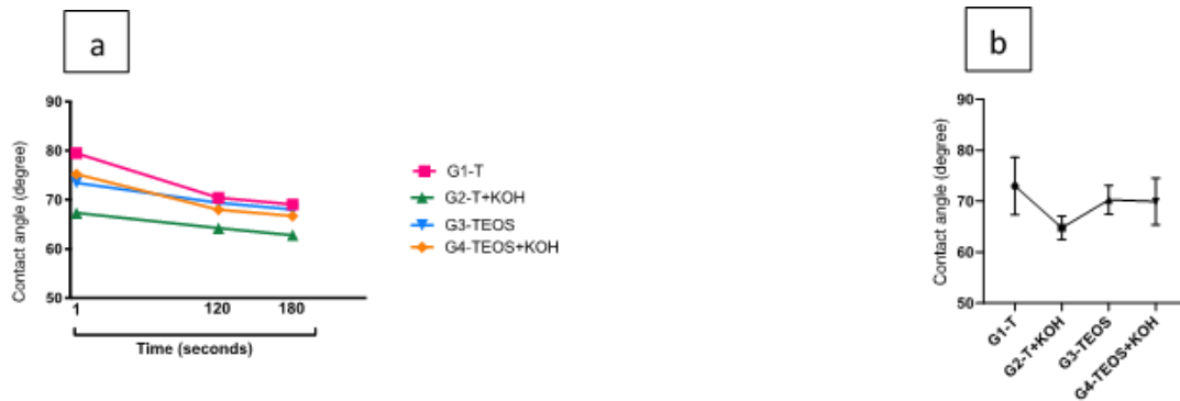
Fig. 3. (a) Contact angle measured at times 1, 120 and 180 seconds. (b) Average contact angle of T, T + KOH, TEOS and TEOS + KOH groups. ANOVA - Tukey's multiple comparisons test ** p > 0.05
