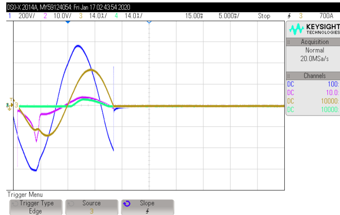
Figure 4.62 Primary (Ch 1 - blue) and secondary (Ch 2 - magenta) voltage, secondary current (Ch 3 - yellow) and i_{T_3} (Ch 4 - cyan) – surge #2.
