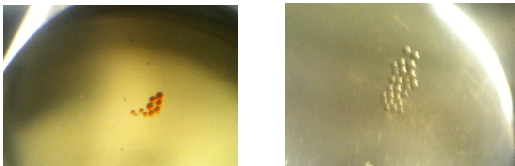
Figure 2.22: Kaiser-test-submitted resin beads color patterns, indicating presence (left) or absence (right) of free amino groups.
