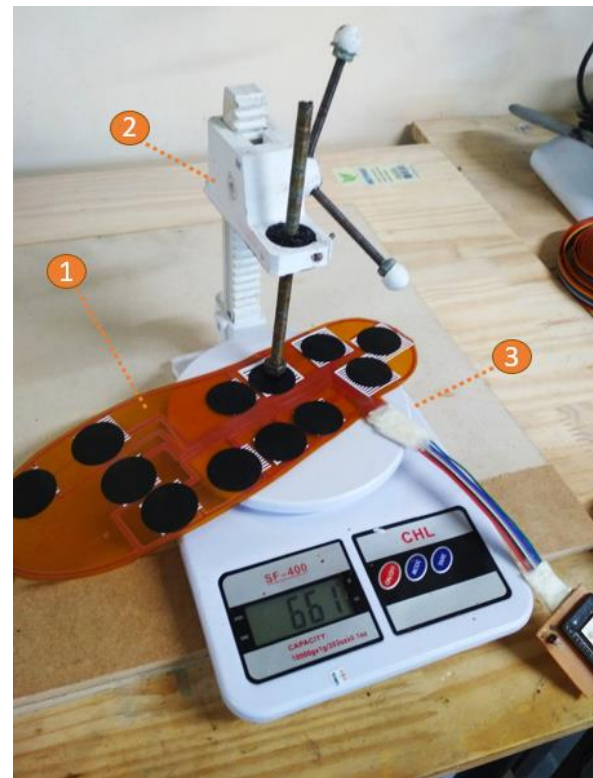
Fig.1. First version and calibration of the sensorized insole.
