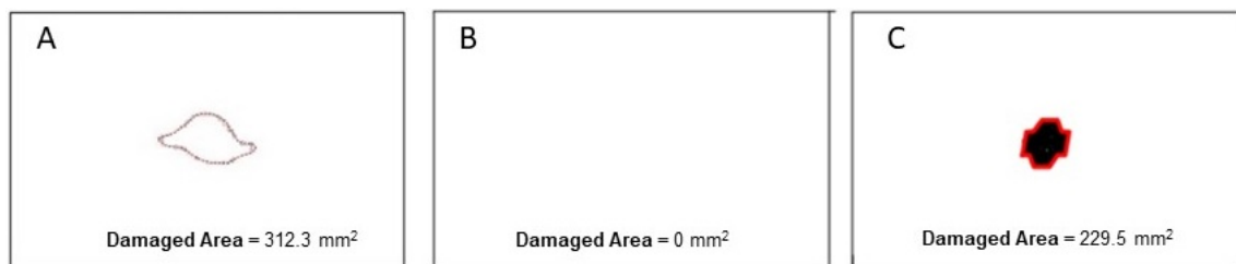
Figure 7.6: Damaged area considering 6.5 J impact: (A) Experimental (Tan et al., 2015a), (B) Case 1: 2D model without cohesive surfaces using native Hashin failure criterion, (C) Case 2: 2D model including cohesive surfaces using native Hashin failure criterion.
