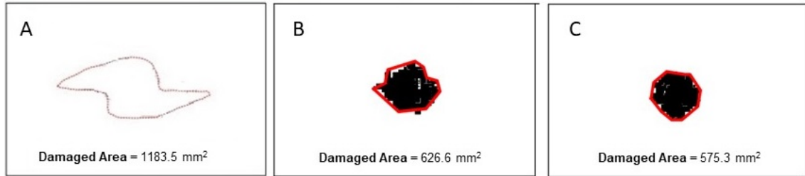
Figure 7.23: Damaged area considering 17 J impact: (A) Experimental (Tan et al., 2015a), (B) Case 3: 3D model including cohesive surfaces using Abaqus available VUMAT with Hashin-Puck-based Nie (2014) failure criterion, (C) Case 4: 3D model including cohesive surfaces using modified VUMAT with Hashin extended failure criterion.
