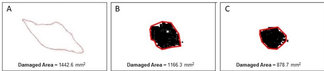
Figure 7.26: Damaged area considering 25 J impact: (A) Experimental (Tan et al., 2015a), (B) Case 3: 3D model including cohesive surfaces using Abaqus available VUMAT with Hashin-Puck-based Nie (2014) failure criterion, (C) Case 4: 3D model including cohesive surfaces using modified VUMAT with Hashin extended failure criterion.
