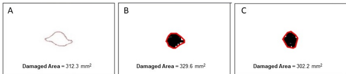
Figure 7.20: Damaged area considering 6.5 J impact: (A) Experimental (Tan et al., 2015a), (B) Case 3: 3D model including cohesive surfaces using Abaqus available VUMAT with Hashin-Puck-based Nie (2014) failure criterion, (C) Case 4: 3D model including cohesive surfaces using modified VUMAT with Hashin extended failure criterion.
