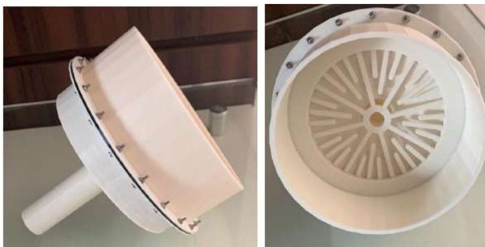
Figure 7 - Prototype of the P02 leaf test filter.
