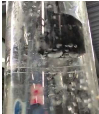
Figure 25 – Bubbles attached to the ultrasonic transducer surface
