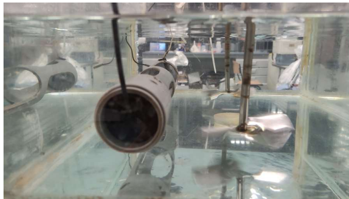
Figure 32 – US sensor inside the setup with water
