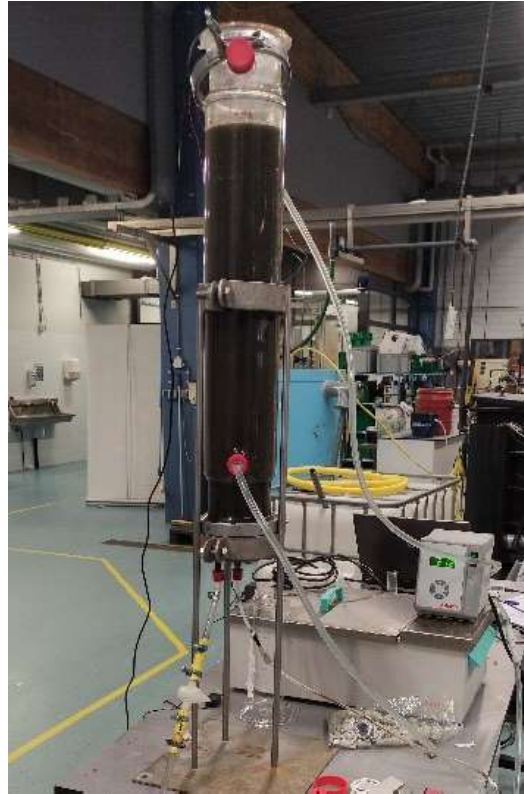
Figure 24 – Vertical reactor with air bubble diffusion
