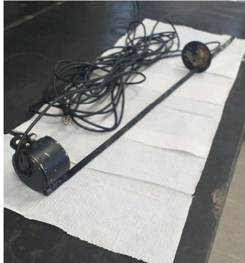
Figure 9 – Transducer case for different distances from the reflection surface
