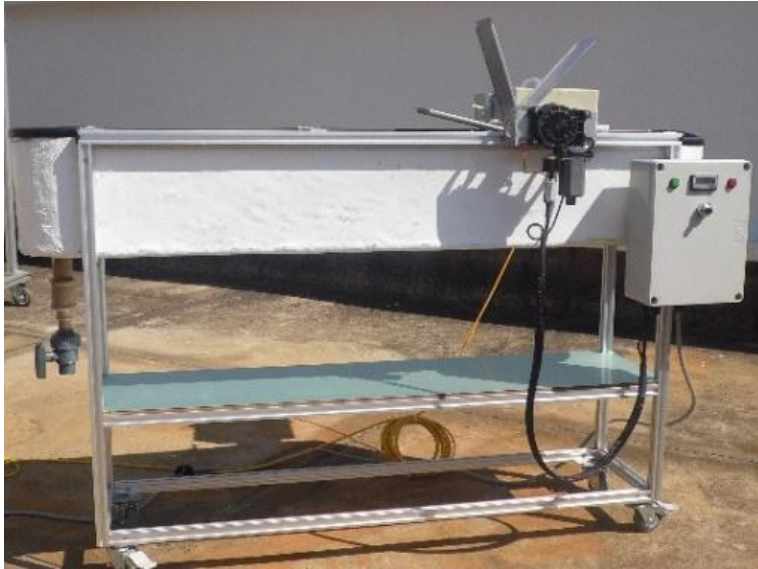
Figure 6.1(a) - RPR reactor (GruPOA).
