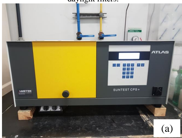
Figure 5.1 – (a) The benchtop solar simulator chamber and (b) the detail of the xenon lamps with daylight filters.
