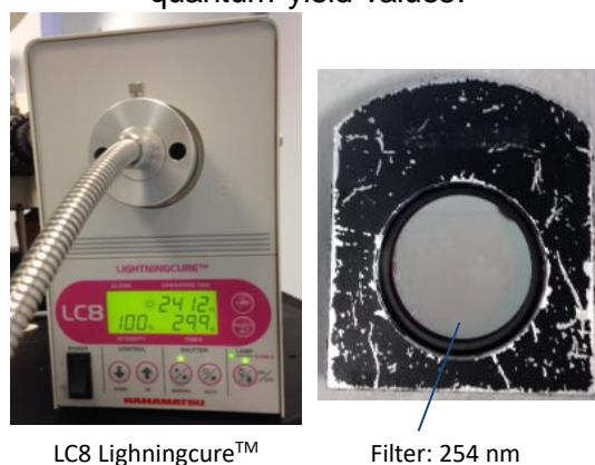
FIGURE 3. 1 – UV-C lamp and filter (254 nm) used in the experiments for the calculation of quantum-yield values.
