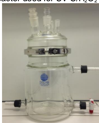
FIGURE 3. 2 – UV-C reactor used for UV-C/H 2 O 2 and UV-C/PS reactions.
