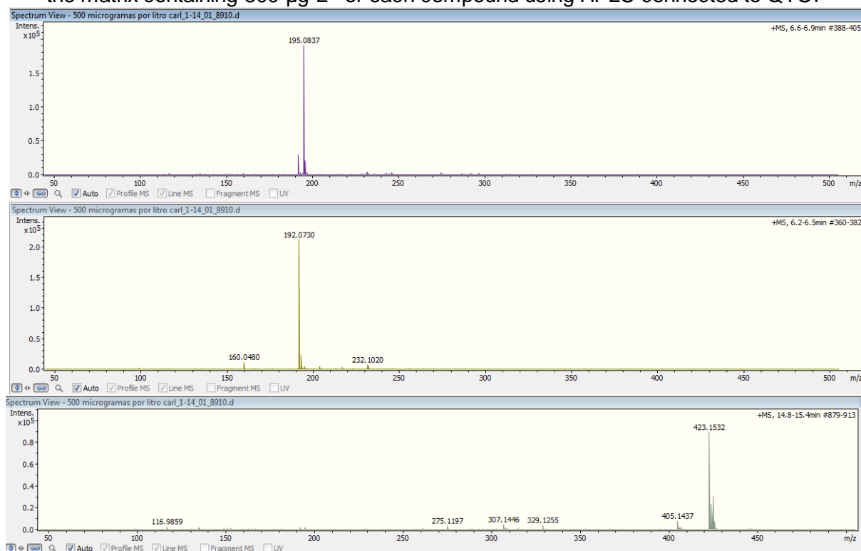
FIGURE 4. 2 – Mass spectrum view of (top) CAF, (center) CBZ and (bottom) LP obtained in the matrix containing 500 µg L -1 of each compound using HPLC connected to QTOF
