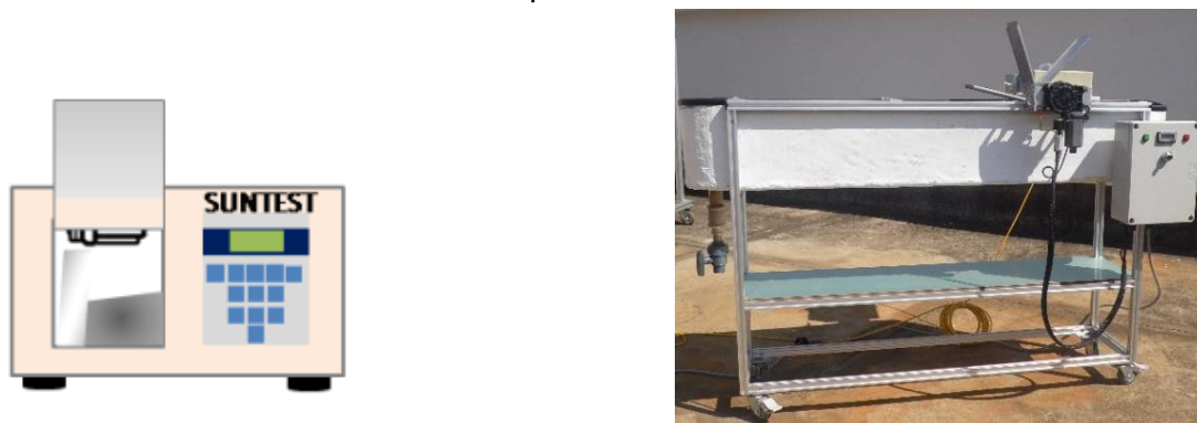
FIGURE 4. 4 - SUNTEST (left) and RPR reactor (right) used for solar photo-Fenton experiments.
