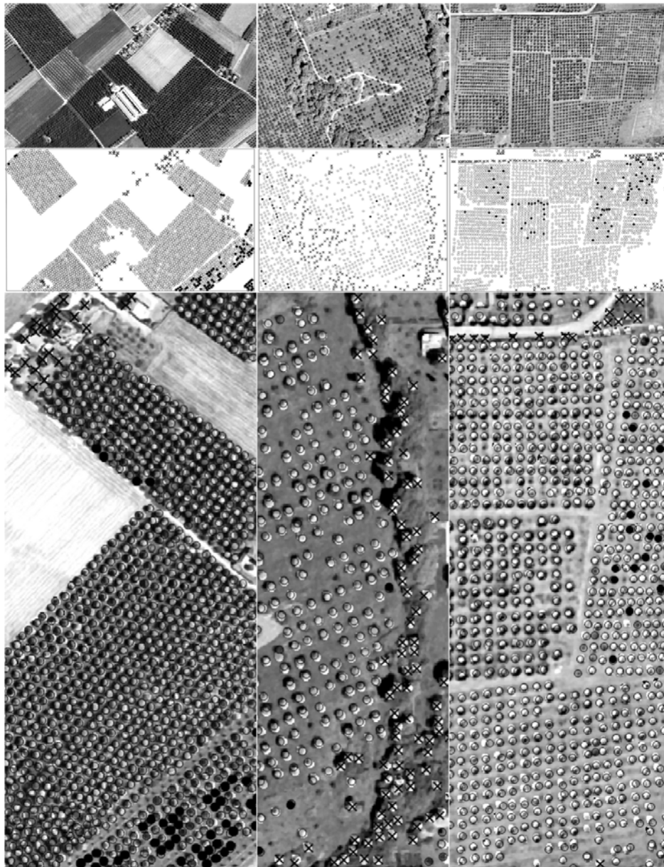
Figure 14. Illustration of the results of the tree counting for the three test images: Grenoble (left column), Briacciano (center column), and Juazeiro (right column). The empty circles represent the trees that were found, “x” represents the false positives and the black circles represent the false negatives.
