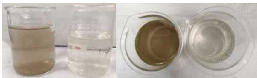
FIGURE III.3.2 – Secondary effluent from the UASB + SBTF system aspect before and after filtration
