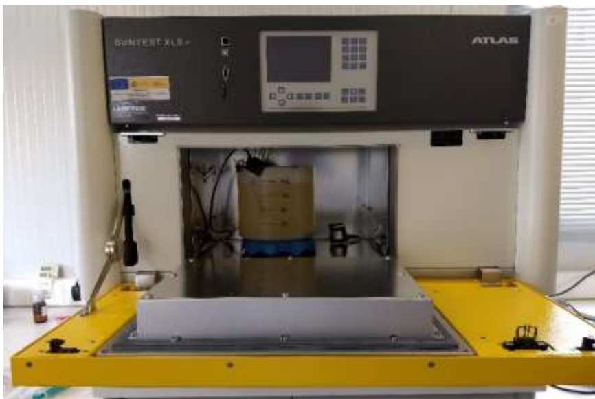
FIGURE II.3.14 – Solar simulator (Sun-Test XLS+, Atlas) equipment used in lab-scale experiments
