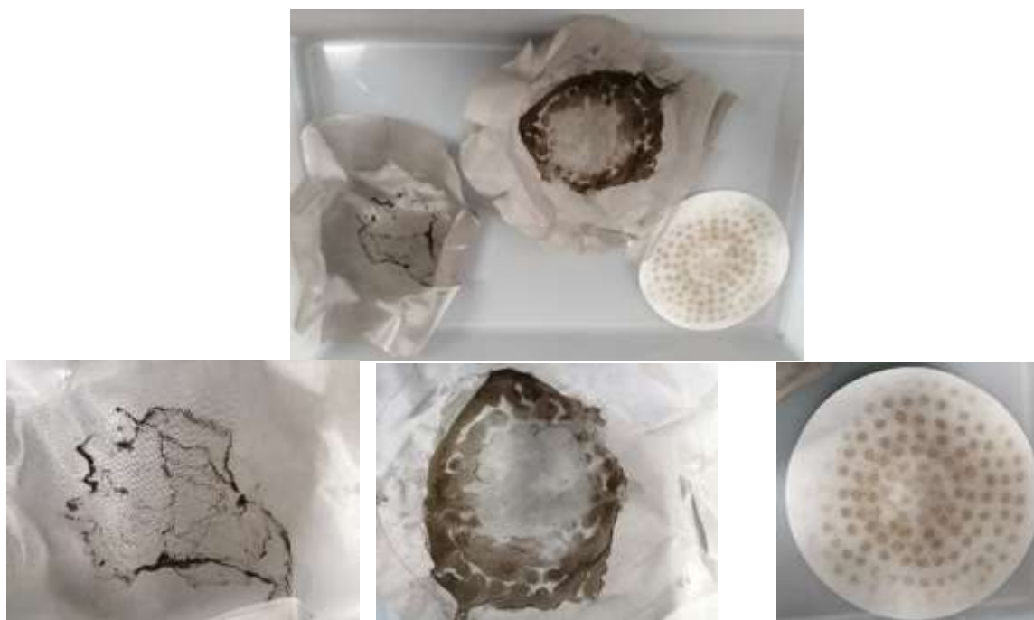
FIGURE III.3.1 – Pre-treatment filtering process: stainless steel mesh filters (100 \mu\text{m} and 5 \mu\text{m} ) and medium flow quantitative paper
