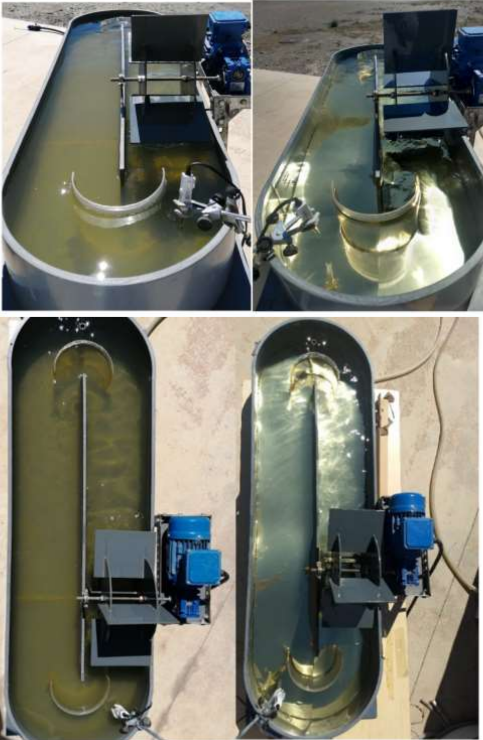
FIGURE II.3.16 – Raceway pond reactors, with and without the aluminum surface on the bottom.
