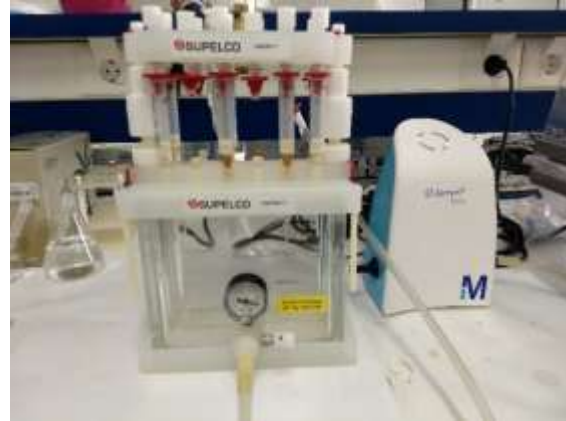
FIGURE II.3.4 – Sample elution with methanol
