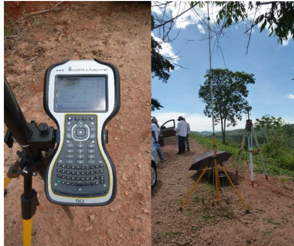
Figure 5. Equipment used to perform RTK geopositioning.
