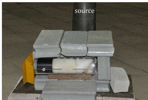
Figure 3 - Rat protected with a covering device at 2 m from the source.
