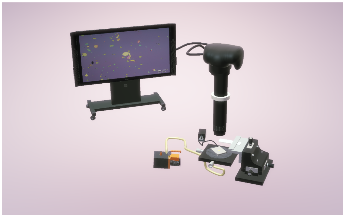
Figure 3.3: Transfer System used to make the vertical stacking of the samples
