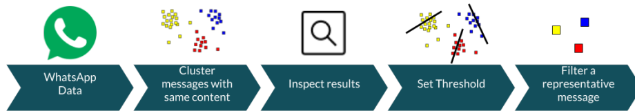
Figure 3.3: Images Filtering Flowchart
