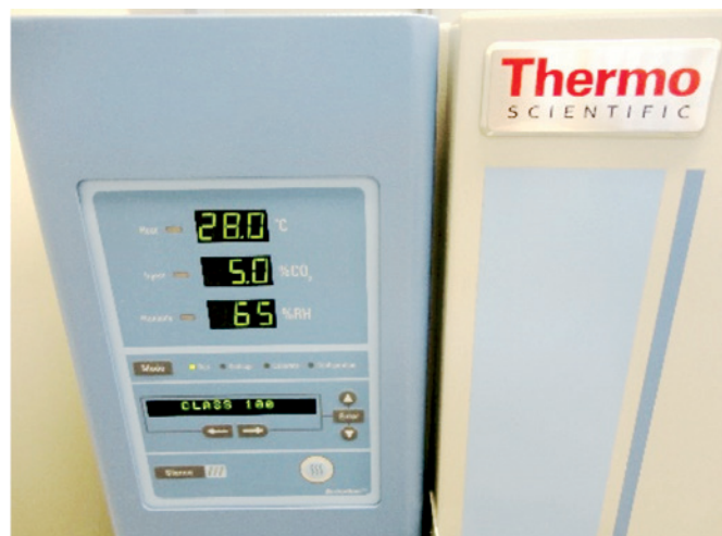
Figure 2 Carbonation chamber – exposure conditions of the specimens
