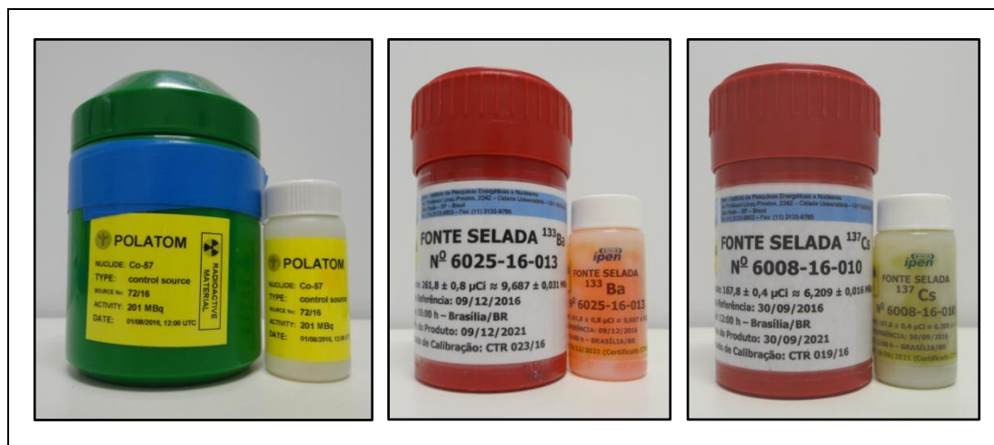
Figure 2: Sealed reference sources for quality control of the activimeter.
