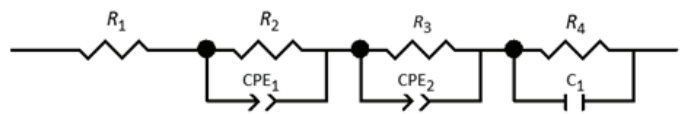
Fig. 3 – Equivalent circuit for steel corrosion in saline solutions with addition of 200 \mu\text{L} and 500 \mu\text{L} of EEP
