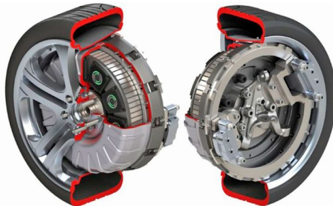
Figure 9 – In-wheel drive solution from Protean ( KLIMOV, 2021 )
