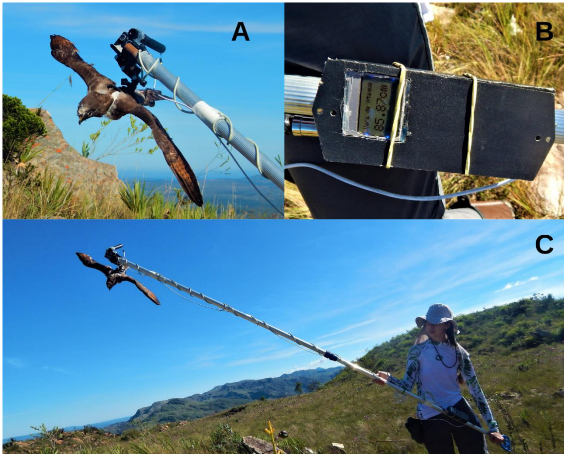
Fig.S1: Pole used during the simulation of a predatory attack on the lizard Eurolophosaurus nanuzae at Serra do Cipó locality, Minas Gerais State, Brazil. A) Taxidermized predator model (hawk Rupornis magnirostris ) attached in typical flight posture at the end of the pole and above the hawk we connected distance sensor to measure the flight initiation distance (FID); B) Display showing the FID estimated by the distance sensor and C) Full view of the pole with the predator model and the electronic system used during the field experiments.
