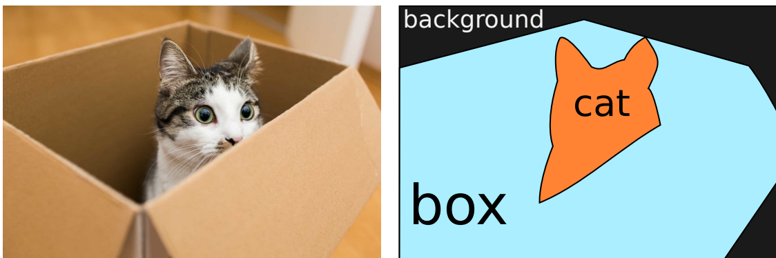
Figure 1.1: Example of semantic segmentation. The image of the cat in the left is segmented, creating 3 semantic groups: cat, box, and background.
