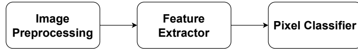
Figure 1 – Common pipeline in semantic segmentation solutions, composed of 1 - an input image preprocessing, 2 - a feature extractor, and 3 - a pixel classifier.
