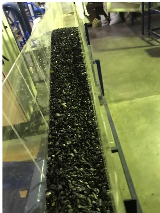
(p) Ensaio 7 -  $Q = 0,91 \text{ L/s}$
