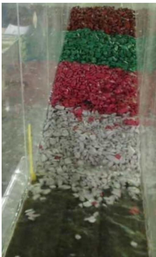
(c)  $Q = 0,28 \text{ L/s}$
