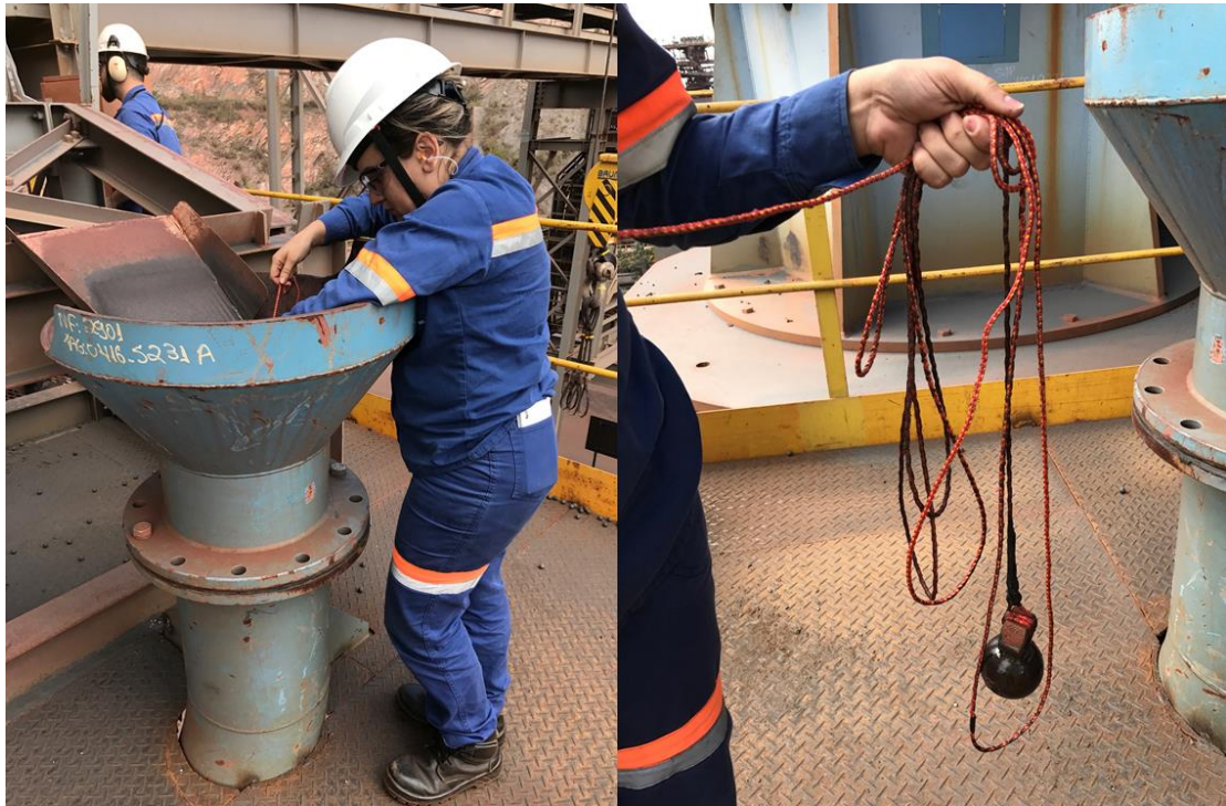
Figure 6.2 – Procedure and equipment for mil filling measurement.
