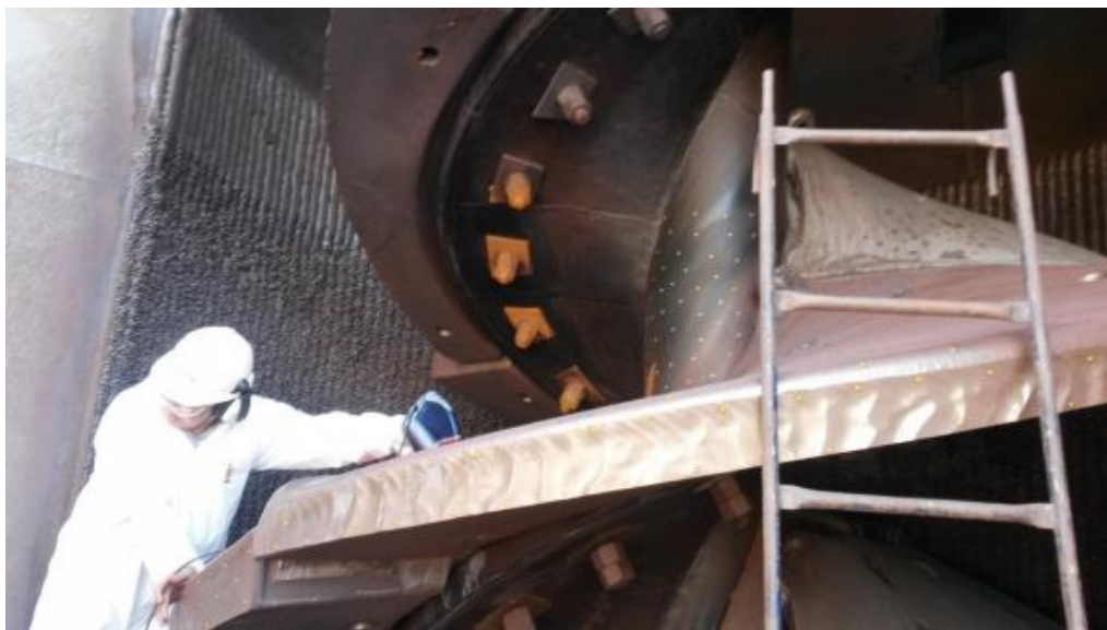
Figure 4.5 - Scanning procedure to obtain three dimensional measurement of liner parts. (Silva, 2019).
