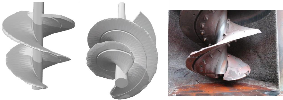
Figure 4.16 - Comparison between 3D worn screw after DEM simulation and industrial worn liner.
