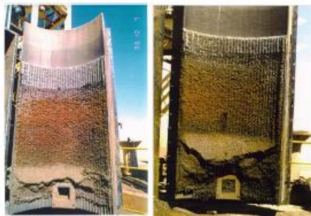
Figure 2.6 – Mill filling at different screw liner wear stages. Left: new liner – Right: worn liner (Allen and Noriega, 2011).
