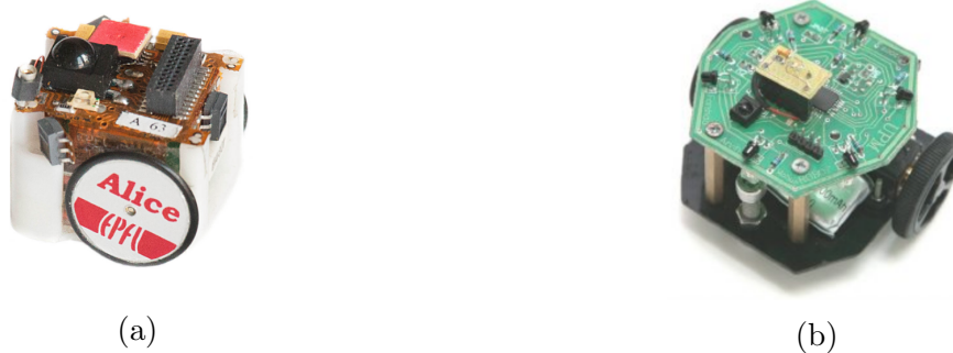
Figure 2.2: An illustration of Alice (a) and AMiR (b) robots. They represent two of the early robots for swarm experimentation
