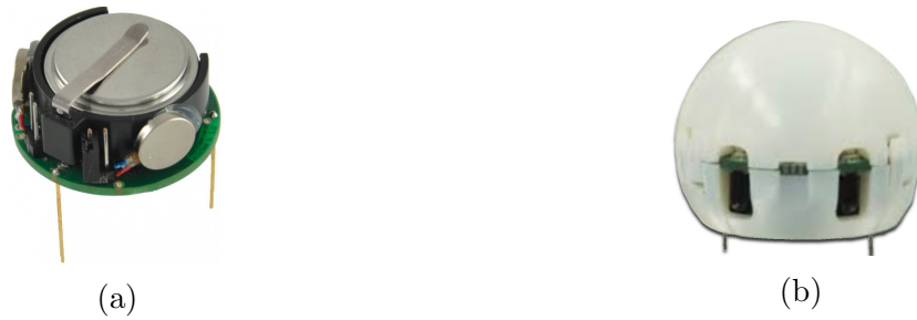
Figure 2.1: An illustration of Kilobot (a) and Droplet (b) robots. They represent two of the latest and more compact platforms for swarm robotics.
