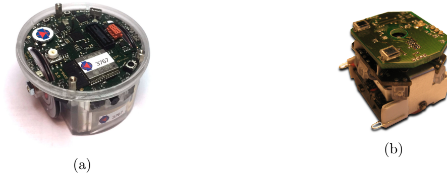
Figure 2.3: An illustration showcasing the E-puck (a) and Jasmine (b) robots is presented. These robots stand as prominent choices extensively employed in swarm research efforts.
