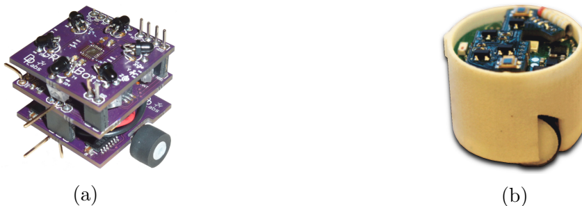
Figure 2.4: An illustrative display featuring the GRITSBot (a) and Zooids (b) robots, two of the most miniature wheeled-based swarm robots.
