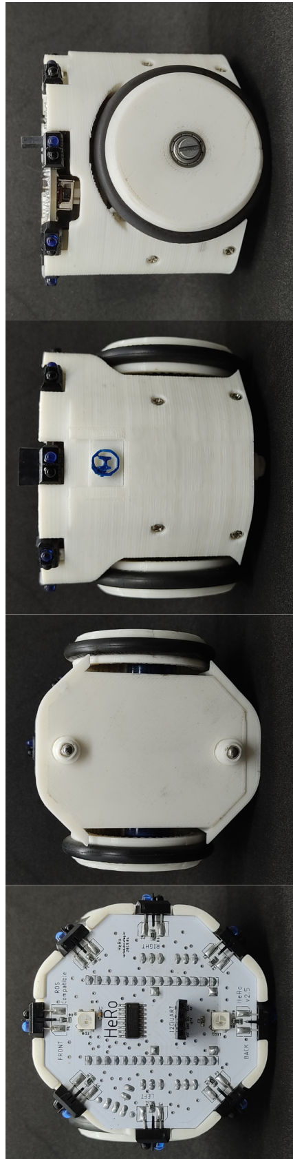
Figure 3.7: Top, bottom, front, and left views of the HeRo swarm platform.
