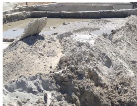
Fig. 3 – Concrete waste bay in batching plants.
