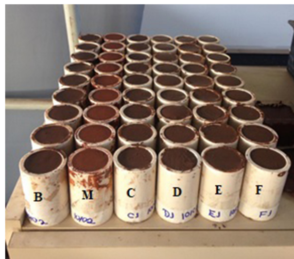
Fig. 1 – Specimens produced (from left to right the rows was classified by B, M, C, D, E and F, being only M a matrix and the others geopolymer).
