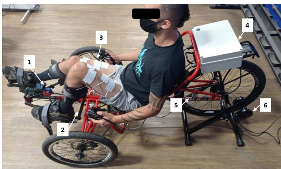
Figure 6. Tadpole tricycle and main components: (1) rotary Encoder, (2) calf support, (3) surface electrodes, (4) proprietary stimulator, (5) speed sensor, (6) cycling trainer.
