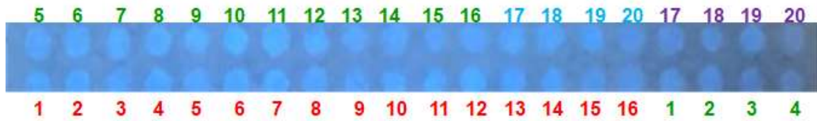
Figure 17 - Cellulose membrane with peptide sequences derived from the rKDDR-plus protein visualized by ultraviolet light. Sixteen peptides selected after the scan were synthesized in sequence on the membrane (numbers 1 to 16 red), and then duplicates of these sequences were synthesized on the membrane (numbers 1 to 16 green). Then, the four sequences containing twelve amino acids each were included in the membrane (numbers 17 to 20 blue), followed by their duplicates (numbers 17 to 20 purple).
